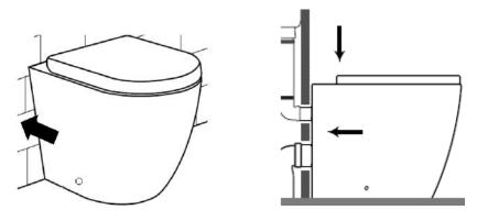
9. Once aligned, secure the toilet pan into position using the fixings provided, do not overtighten. Finish by pushing on the screw covers.
