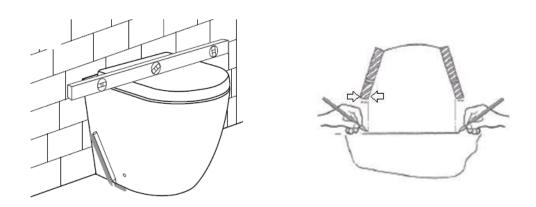
4. Remove the pan from the location, turn over, then measure the thickness of the toilet side wall and make another mark in from the original mark, and in line with the fixing hole, as shown below. Repeat on the other side.
